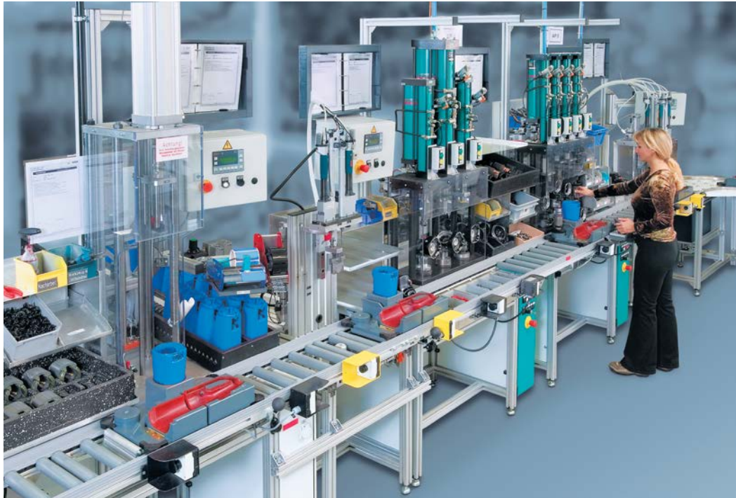
Assembly and test stands for precision cordless screwdrivers
