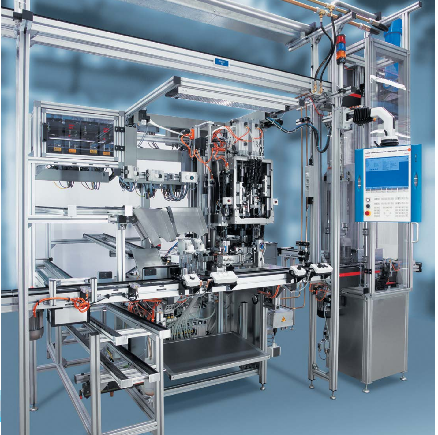
Flexible line with transfer system and manual supply
