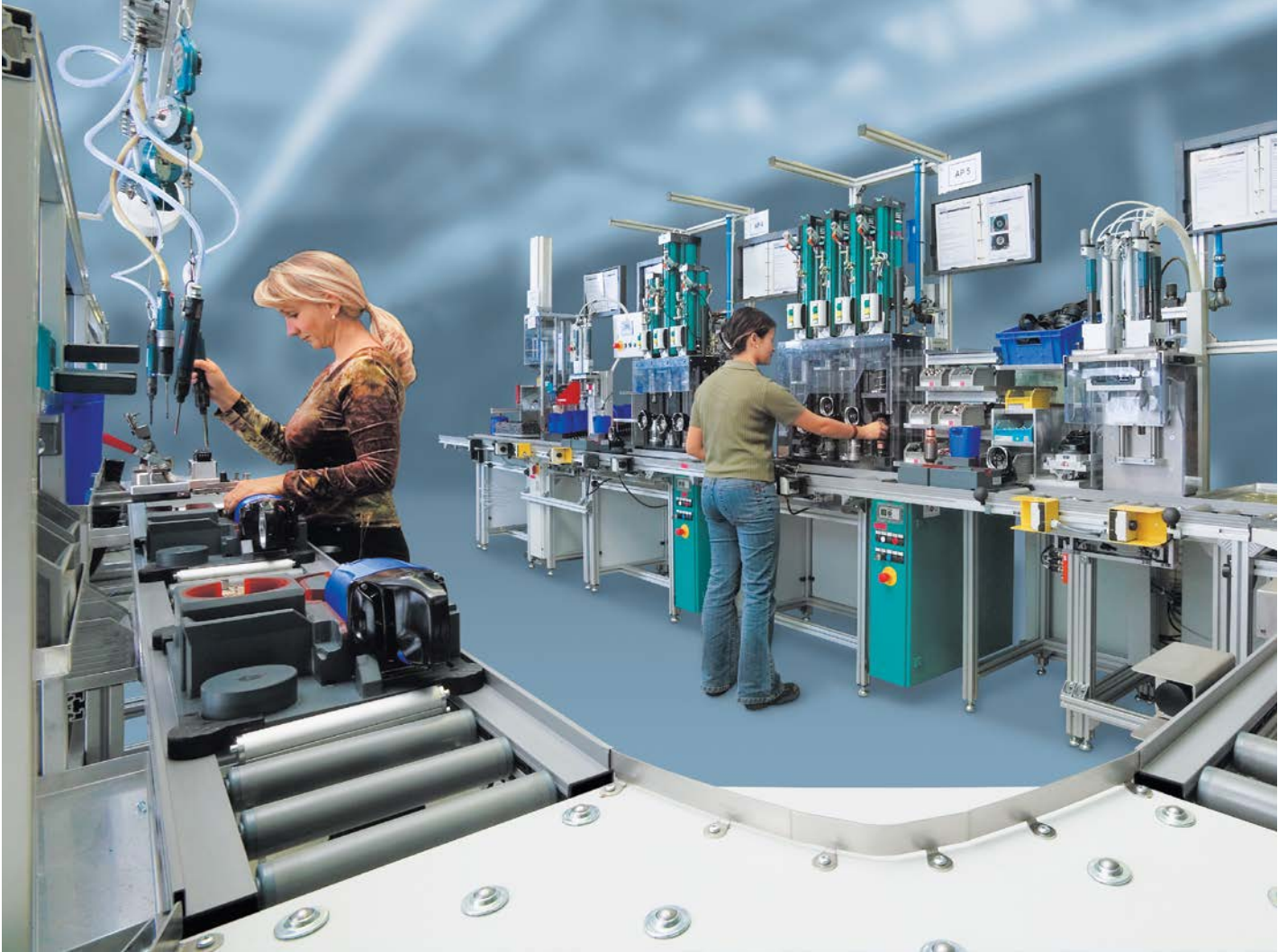
Lean production with manual process linking for angle grinder production
