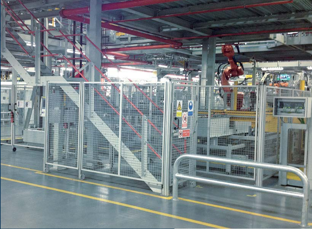
Fully automatic body assembly with the EcoSafe protective fence
