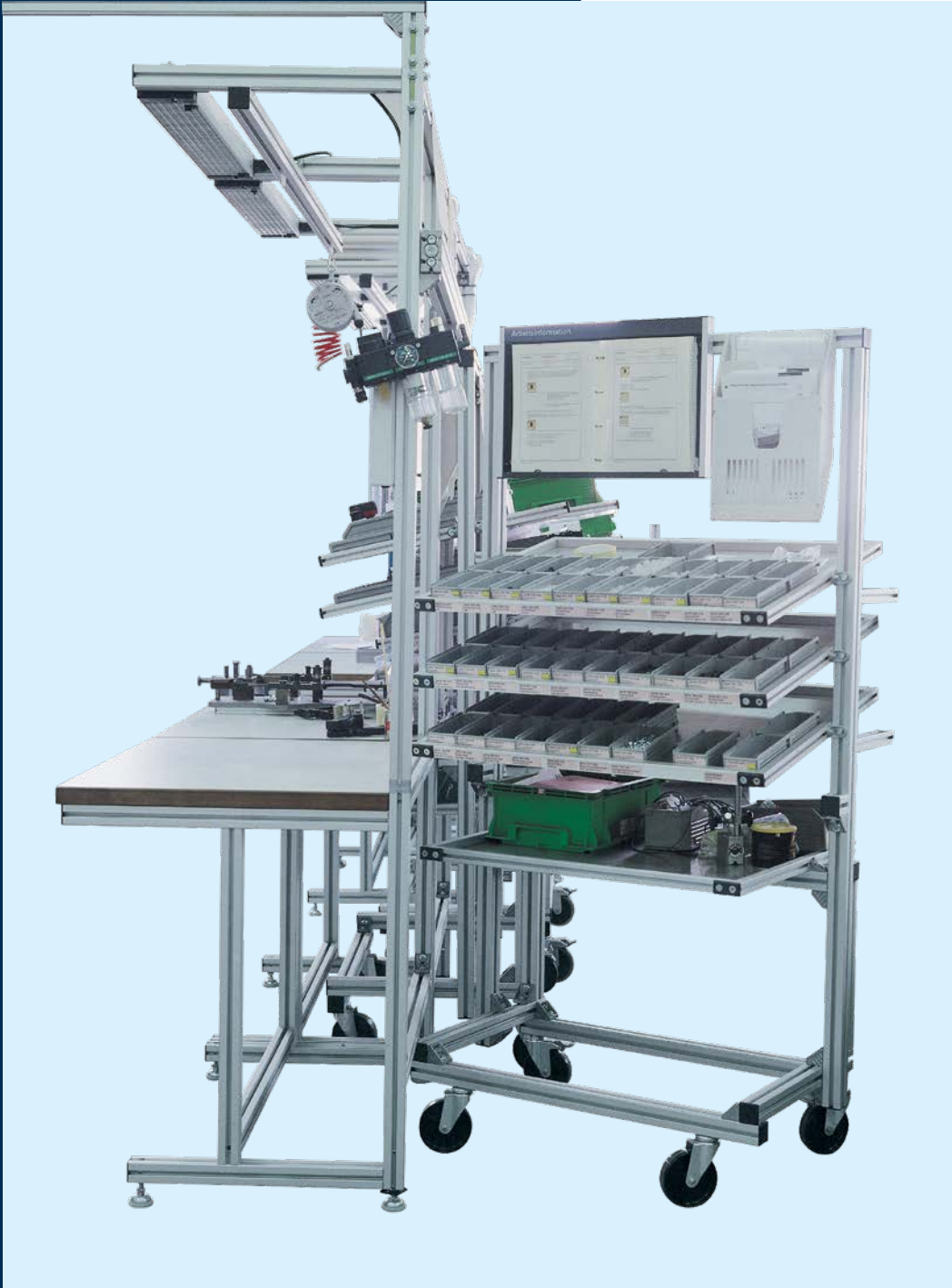
Flexible workstation with dockable material shuttle
