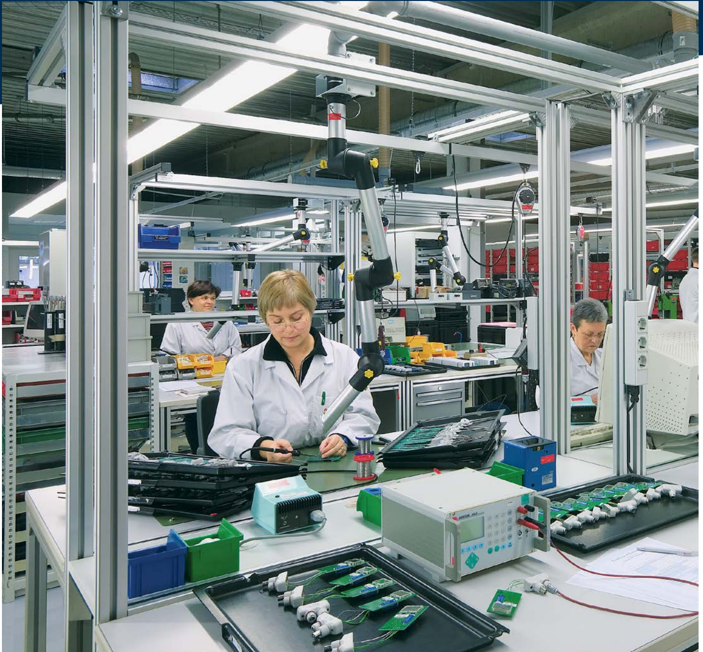
ESD assembly of water-proof temperature sensors
