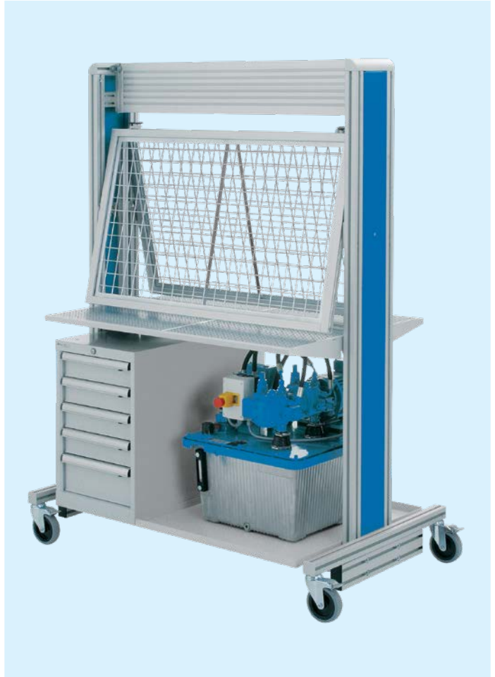
Tightening station for alternator production
