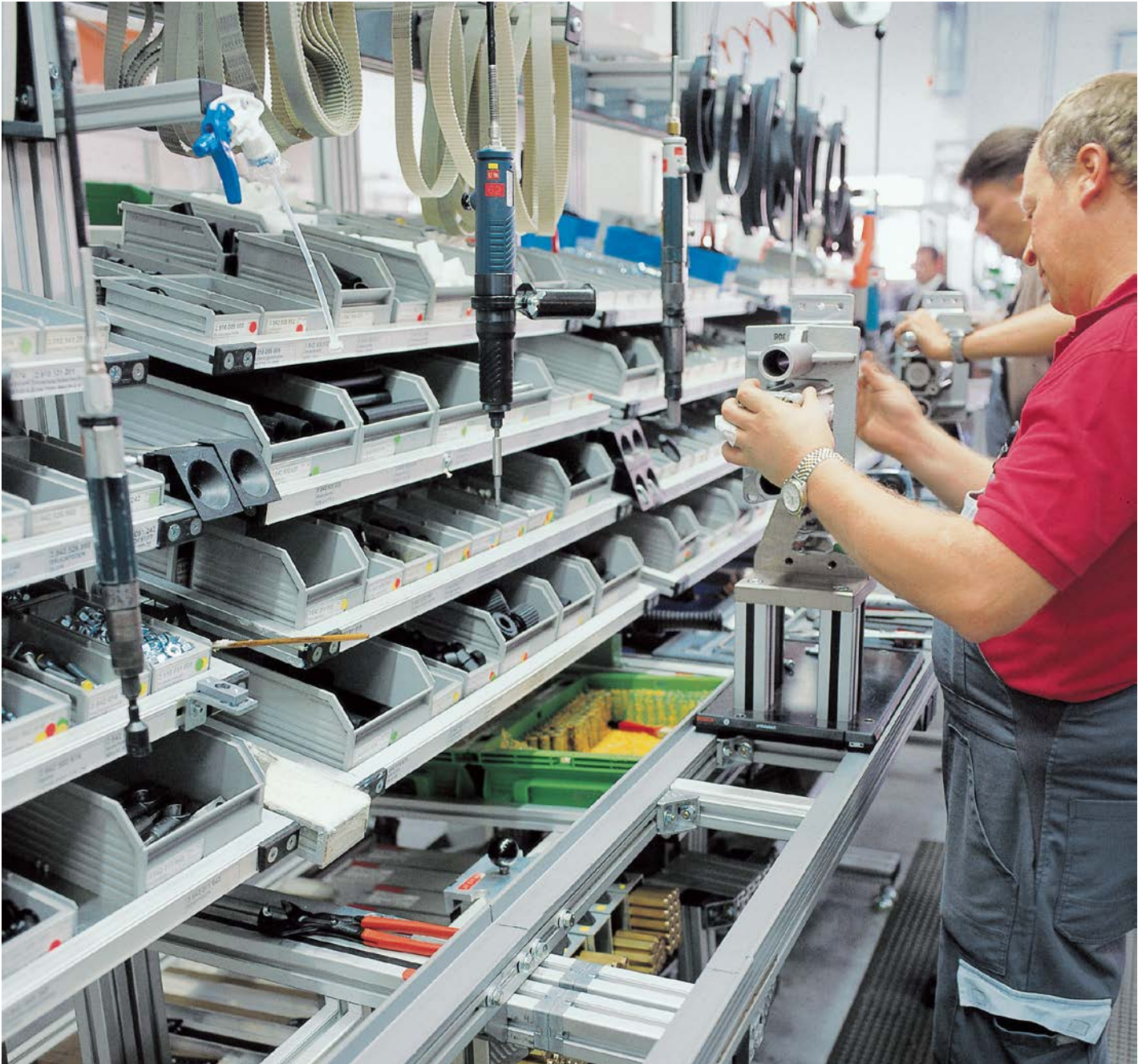
Lean production with manual process linking
