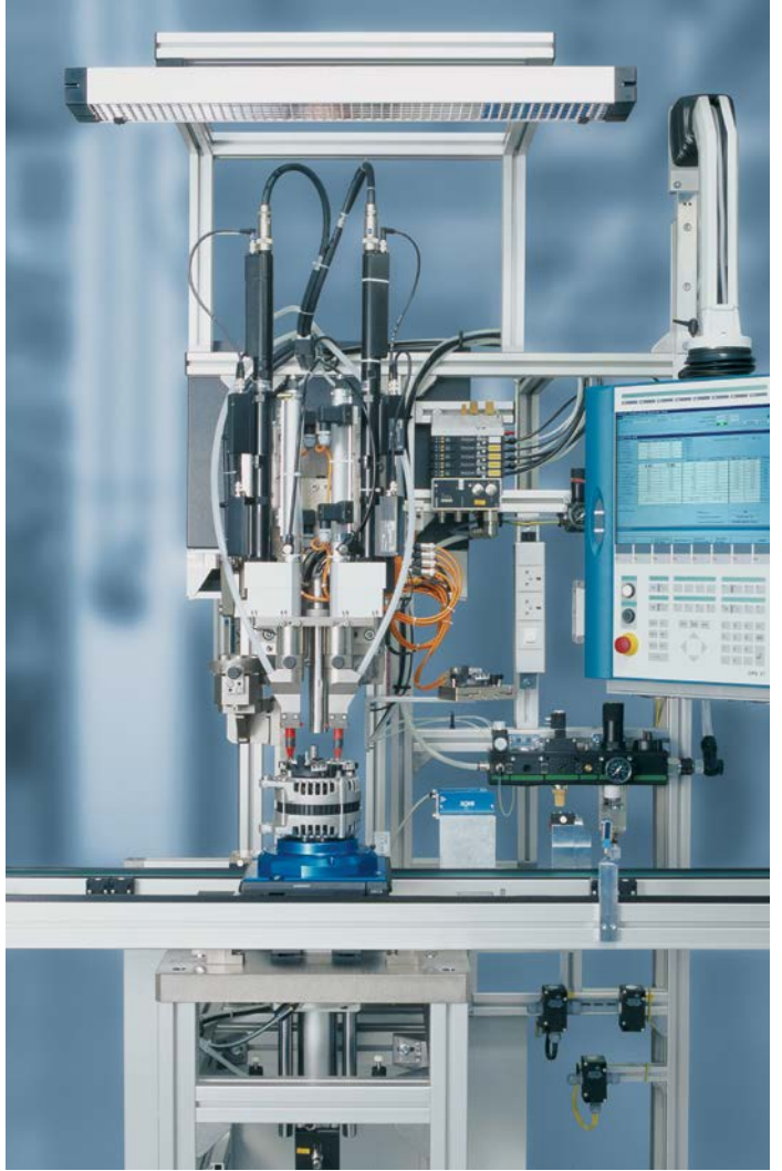
Tightening station for alternator production
