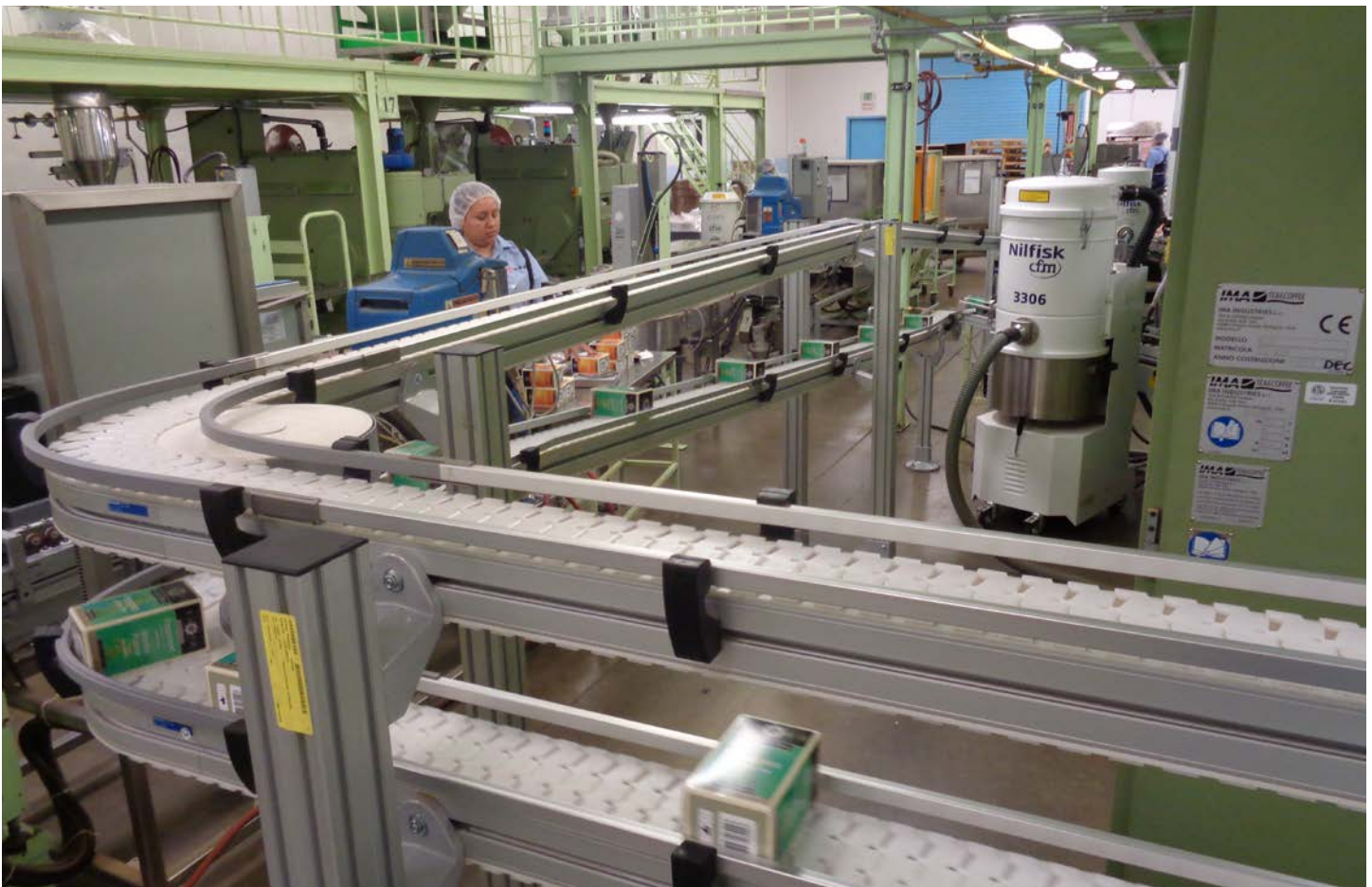
VarioFlow plus was varied through the use of vertical inclines and lateral off-sets to achieve a stacked configuration, allowing for a very narrow footprint.
