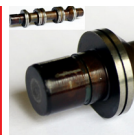
Valve piston with deposits
