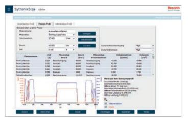
By means of SytronixSize, hydraulic and electrical components can be dimensioned on the basis of application-specific specifications. As all product-relevant data and models are contain, the design process is automated.
