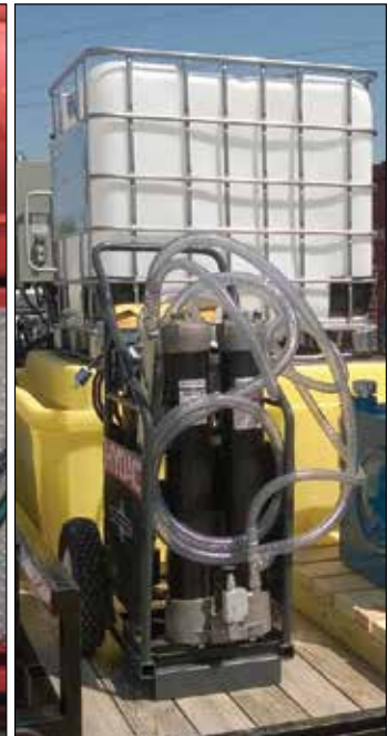
OFS Filtration Station with HPU.
