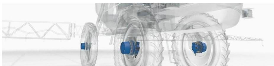
Especially in agricultural sprayers, the advantages of the internal multi-disc brake come fully to bear. It is lighter in weight than conventional designs and its protection against grime greatly reduces the need for maintenance.
