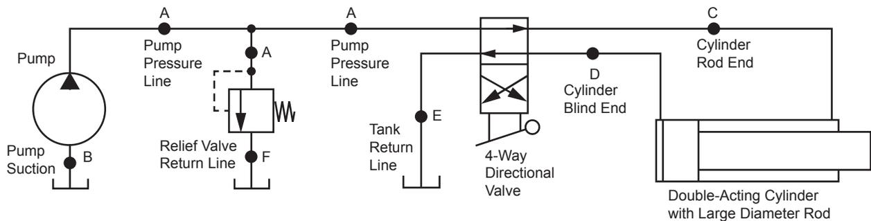
**Figure 1.** In different parts of the hydraulic circuit, flows and pressures are different. The optimum piping size for each line can be determined from permissible flow velocity and available pressure in each line
