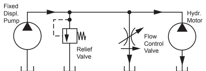
*Figure 1. By-pass method of motor speed control.*
