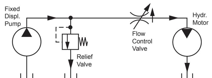
*Figure 2. Series meter-in method of motor speed control.*
