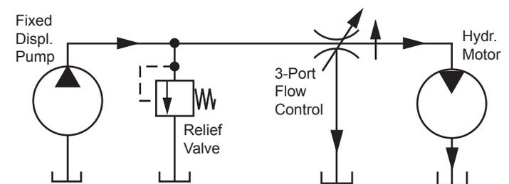
*Figure 3. Three-port flow control method.*
