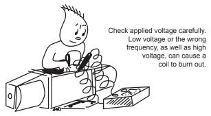
c. **Frequency.** Operation of a 60 Hz coil on 50 Hz causes the coil to draw above normal current. Operation of a 50 Hz coil on 60 Hz causes the coil to draw less than rated current and it may burn out from inability to pull in.
